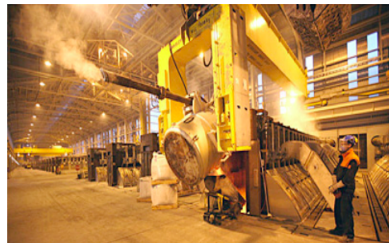
Figure 17: Hazardous conditions in an aluminium pot room a .
